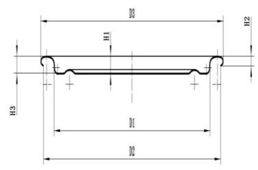
The outer diameter of the rolling edge (D3) is  $72.20\pm0.10$ mm Inner diameter of flange (D2)  $70.40\pm0.30$ mm Flange height (H2)  $1.95\pm0.10$ Buried depth (H3)  $3.00\pm0.10$ mm Can diameter (D1)  $62.35\pm0.10$ mm Indenter fits well with the company's indenter Thickness of iron sheet 0.19-0.20Iron hardness T4CA/T4BA
