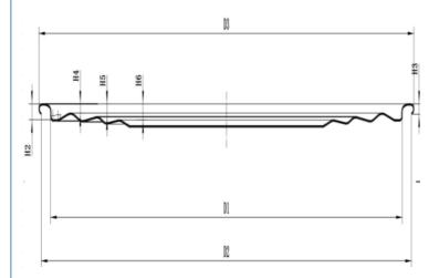
The outer diameter of the flange (D3) is 93.20±0.20mm Inner diameter of flange (D2) 91.20±0.30mm Flange height (H3) 1.95±0.10 Buried depth (H2) 3.00±0.10mm Can diameter (D1) 83.30±0.10mm Dry glue quantity 70-90mg Moisture content ≤3% Indenter fits well with the company's indenter
