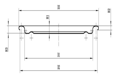
Outer diameter of rolling edge (D3) 61.15±0.15mm Inner diameter of flange (D2) 59.60±0.30mm Flange height (H2) 1.95±0.10 Buried depth (H3) 3.00±0.10mm Fit diameter (D1) 52.30±0.10mm Indenter fits well with the company's indenter
