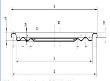
Outer diameter of rolling edge (D3) 82.50±0.10mm Inner diameter of flange (D2) 81.10±0.30mm Flange height (H2) 1.95±0.10 Buried depth (H3) 2.9500±0.20mm Can diameter (D1) 73.00±0.10mm Indenter fits well with the company's indenter Thickness of iron sheet 0.17-0.18 Iron hardness T4CA/T4BA Coated with gloss oil/gold oil Inner coating oil/gold oil/white porcelain, yellow porcelain
