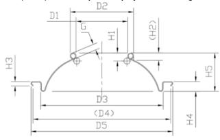
Outer diameter (D5) 64.40±0.20mm Inner diameter of flange (D4) 62.0±0.20mm Flange height (H3) 2.45±0.15mm Buried depth (H4) 4.80±0.20mm Total height (H5) 17.20±0.2mm Contact height (H1) 4.00±0.10mm Fit diameter (D3) / Outer diameter of tank mouth (D2) 31.20±0.10mm Inside diameter of tank mouth (D1) 25.40±0.10mm Dry glue quantity 75-95mg
