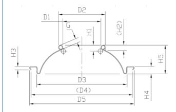
Flange diameter (D5) 57.60±0.20mm Inner diameter of flange (D4) 55.70±0.20mm Flange height (H3) 2.20±0.15mm Buried depth (H4) 4.70±0.15mm Total height (H5) 13.50±0.15mm Contact height (H1) 4.00±0.10mm Fit diameter (D3) 48.00±0.20mm Outer diameter of tank mouth (D2) 31.20±0.10mm
