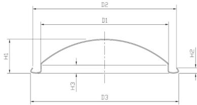
Flange diameter (D3) 67.2±0.25mm Inner diameter of flange (D2) 65.20±0.25mm Flange height (H2) 2.30±0.2mm Dry glue quantity 70-90mg
