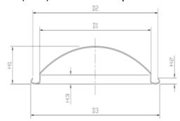
The outer diameter of the flange (D3) is 75.00±0.20mm Inner diameter of flange (D2) 73.10±0.30mm Flange height (H2) 2.45±0.15 Buried depth (H3) 3.10±0.15mm Total covering height (H1) 14.70±0.20mm Fit diameter (D1) 65.10±0.20mm Dry glue quantity 90-110mg Deformation pressure ≥1.3MPa Bursting pressure ≥1.5MPa Indenter fits well with the company's indenter Thickness of iron sheet 0.32-0.33
