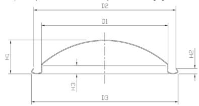
The outer diameter of the flange (D3) is 72.35±0.25mm
