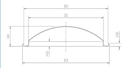
The outer diameter of the flange (D3) is  $72.35\pm0.25$ mm Inner diameter of flange (D2)  $70.00\pm0.25$ mm Flange height (H2)  $2.50\pm0.2$ mm Buried depth (H3)  $3.10\pm0.15$ mm Fit diameter (D1)  $62.80\pm0.20$ mm Dry glue quantity 70-90mg Deformation pressure  $\geq 1.8$ MPa Burst pressure  $\geq high$  pressure 2.1MPa Indenter fits well with the company's indenter Sheet thickness 0.4 Iron hardness T4CA
