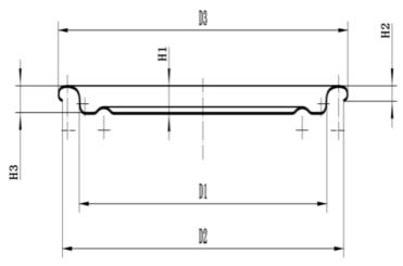
The outer diameter of the rolling edge (D3) is 72.20±0.10mm Inner diameter of flange (D2) 70.40±0.30mm Flange height (H2) 1.95±0.10 Buried depth (H3) 3.00±0.10mm Can diameter (D1) 62.35±0.10mm Indenter fits well with the company's indenter Thickness of iron sheet 0.19-0.20 Iron hardness T4CA/T4BA
