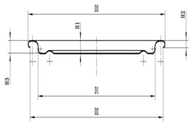
The outer diameter of the rolling edge (D3) is  $59.05\pm0.20$ mm Inner diameter of flange (D2)  $57.40\pm0.30$ mm Flange height (H2)  $1.95\pm0.10$ Buried depth (H3)  $3.00\pm0.10$ mm Fit diameter (D1)  $49.80\pm0.10$ mm Indenter fits well with the company's indenter Iron sheet thickness 0.18-0.20Iron hardness T4CA/T4BA
