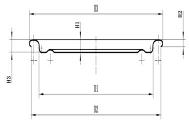
The outer diameter of the rolling edge (D3) is 59.05±0.20mm Inner diameter of flange (D2) 57.40±0.30mm Flange height (H2) 1.95±0.10 Buried depth (H3) 3.00±0.10mm Fit diameter (D1) 49.80±0.10mm Indenter fits well with the company's indenter Iron sheet thickness 0.18-0.20 Iron hardness T4CA/T4BA
