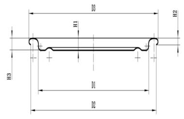
The outer diameter of the rolling edge (D3) is 59.05±0.20mm Inner diameter of flange (D2) 57.40±0.30mm Flange height (H2) 1.95±0.10 Buried depth (H3) 3.00±0.10mm
