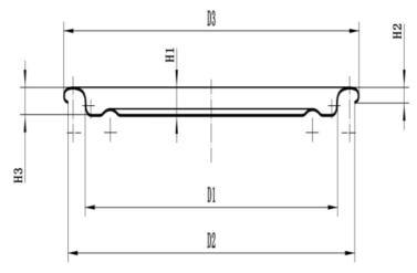
The outer diameter of the rolling edge (D3) is 59.05±0.20mm Inner diameter of flange (D2) 57.40±0.30mm Flange height (H2) 1.95±0.10 Buried depth (H3) 3.00±0.10mm Fit diameter (D1) 49.80±0.10mm Indenter fits well with the company's indenter Iron sheet thickness 0.18-0.20 Iron hardness T4CA/T4BA
