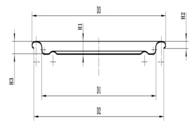
Outer diameter of rolling edge (D3) 61.15±0.15mm Inner diameter of flange (D2) 59.60±0.30mm Flange height (H2) 1.95±0.10 Buried depth (H3) 3.00±0.10mm Fit diameter (D1) 52.30±0.10mm Indenter fits well with the company's indenter
