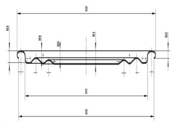
Outer diameter of rolling edge (D3) 82.50±0.10mm Inner diameter of flange (D2) 81.10±0.30mm Flange height (H2) 1.95±0.10 Buried depth (H3) 2.9500±0.20mm Can diameter (D1) 73.00±0.10mm Indenter fits well with the company's indenter
