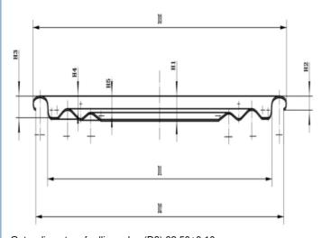
Outer diameter of rolling edge (D3) 82.50±0.10mm Inner diameter of flange (D2) 81.10±0.30mm Flange height (H2) 1.95±0.10 Buried depth (H3) 2.9500±0.20mm Can diameter (D1) 73.00±0.10mm Indenter fits well with the company's indenter Thickness of iron sheet 0.17-0.18 Iron hardness T4CA/T4BA
