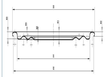
Outer diameter of rolling edge (D3) 82.50±0.10mm Inner diameter of flange (D2) 81.10±0.30mm Flange height (H2) 1.95±0.10 Buried depth (H3) 2.9500±0.20mm Can diameter (D1) 73.00±0.10mm Indenter fits well with the company's indenter Thickness of iron sheet 0.17-0.18 Iron hardness T4CA/T4BA
