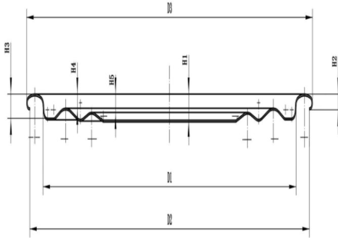
Outer diameter of rolling edge (D3)  $82.50 \pm 0.10$ mm
