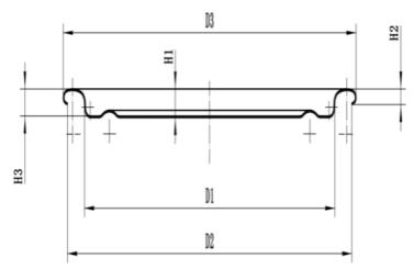
The outer diameter of the rolling edge (D3) is  $72.20\pm0.10$ mm Inner diameter of flange (D2)  $70.40\pm0.30$ mm Flange height (H2)  $1.95\pm0.10$ Buried depth (H3)  $3.00\pm0.10$ mm Can diameter (D1)  $62.35\pm0.10$ mm Indenter fits well with the company's indenter Thickness of iron sheet 0.19-0.20Iron hardness T4CA/T4BA
