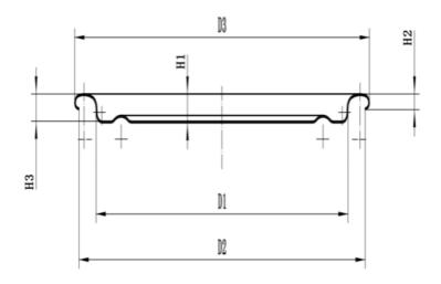
The outer diameter of the rolling edge (D3) is 72.20±0.10mm Inner diameter of flange (D2) 70.40±0.30mm Flange height (H2) 1.95±0.10 Buried depth (H3) 3.00±0.10mm Can diameter (D1) 62.35±0.10mm Indenter fits well with the company's indenter Thickness of iron sheet 0.19-0.20 Iron hardness T4CA/T4BA
