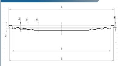
The outer diameter of the flange (D3) is 163.70±0.10mm Inner diameter of flange (D2) 162.00±0.30mm Flange height (H3) 2.10±0.10 Buried depth (H2) 3.40±0.10mm Fit diameter (D1) 153.50±0.10mm Indenter fits well with the company's indenter Thickness of iron sheet 0.23-0.24 Iron hardness T4CA/T4BA
