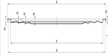
The outer diameter of the flange (D3) is  $163.70\pm0.10$ mm Inner diameter of flange (D2)  $162.00\pm0.30$ mm Flange height (H3)  $2.10\pm0.10$ Buried depth (H2)  $3.40\pm0.10$ mm Fit diameter (D1)  $153.50\pm0.10$ mm Indenter fits well with the company's indenter Thickness of iron sheet 0.23-0.24Iron hardness T4CA/T4BA
