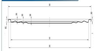
The outer diameter of the flange (D3) is 163.70±0.10mm Inner diameter of flange (D2) 162.00±0.30mm Flange height (H3) 2.10±0.10 Buried depth (H2) 3.40±0.10mm Fit diameter (D1) 153.50±0.10mm Indenter fits well with the company's indenter Thickness 0.23-0.24mm Iron hardness T4CA/T4BA
