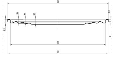
The outer diameter of the flange (D3) is 163.70±0.10mm Inner diameter of flange (D2) 162.00±0.30mm Flange height (H3) 2.10±0.10 Buried depth (H2) 3.40±0.10mm Fit diameter (D1) 153.50±0.10mm Indenter fits well with the company's indenter Thickness of iron sheet 0.23-0.24 Iron hardness T4CA/T4BA
