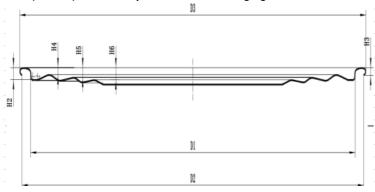
The outer diameter of the flange (D3) is 163.70±0.10mm Inner diameter of flange (D2) 162.00±0.30mm Flange height (H3) 2.10±0.10 Buried depth (H2) 3.40±0.10mm Fit diameter (D1) 153.50±0.10mm Indenter fits well with the company's indenter Thickness of iron sheet 0.23-0.24 Iron hardness T4CA/T4BA
