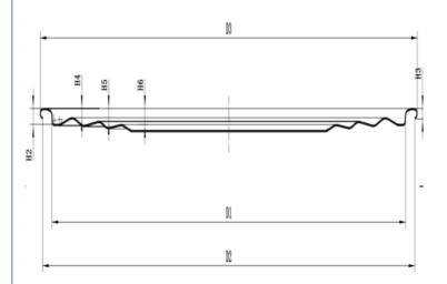
The outer diameter of the flange (D3) is  $93.20\pm0.20$ mm Inner diameter of flange (D2)  $91.20\pm0.30$ mm Flange height (H3)  $1.95\pm0.10$ Buried depth (H2)  $3.00\pm0.10$ mm Can diameter (D1)  $83.30\pm0.10$ mm Dry glue quantity 70-90mg Moisture content  $\leq 3\%$ Indenter fits well with the company's indenter
