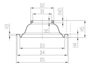
Outer diameter of the flange (D5) 75.50±0.20mm Inner diameter of flange (D4) 73.10±0.30mm Flange height (H3) 2.35±0.15
