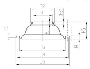
Outer diameter of the flange (D5) 75.50±0.20mm Inner diameter of flange (D4) 73.10±0.30mm Flange height (H3) 2.35±0.15 Buried depth (H4) 4.90±0.15mm Total height (H5) 25.00±0.20mm Contact height (H1) 4.00±0.10mm Fit diameter (D3) 65.30±0.20mm Outer diameter of tank mouth (D2) 31.20±0.10mm Inside diameter of tank mouth (D1) 25.40±0.10mm Dry glue quantity 90-110mg Deformation pressure ≥1.3MPa Bursting pressure ≥1.5MPa Indenter fits well with the company's indenter
