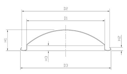
The outer diameter of the flange (D3) is 72.35 $\pm$ 0.25mm Inner diameter of flange (D2) 70.00 $\pm$ 0.25mm Flange height (H2) 2.50 $\pm$ 0.2mm Buried depth (H3) 3.10 $\pm$ 0.15mm Fit diameter (D1) 62.80 $\pm$ 0.20mm Dry glue quantity 70-90mg Deformation pressure  $\geq$  1.8MPa Burst pressure  $\geq$  high pressure 2.1MPa Indenter fits well with the company's indenter Sheet thickness 0.4 Iron hardness T4CA
