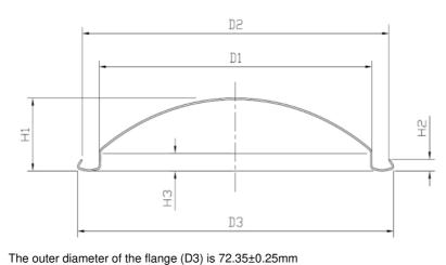
Inner diameter of flange (D2) 70.00±0.25mm Flange height (H2) 2.50±0.2mm Buried depth (H3) 3.10±0.15mm Fit diameter (D1) 62.80±0.20mm Dry glue quantity 70-90mg Deformation pressure ≥ 1.8MPa Burst pressure ≥ high pressure 2.1MPa Indenter fits well with the company's indenter Sheet thickness 0.4
