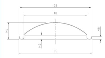
The outer diameter of the flange (D3) is  $72.35\pm0.25$ mm Inner diameter of flange (D2)  $70.00\pm0.25$ mm Flange height (H2) 2.50±0.2mm Buried depth (H3) 3.10±0.15mm Fit diameter (D1) 62.80±0.20mm Dry glue quantity 70-90mg Deformation pressure ≥ 1.8MPa Burst pressure ≥ high pressure 2.1MPa Indenter fits well with the company's indenter Sheet thickness 0.4 Iron hardness T4CA
