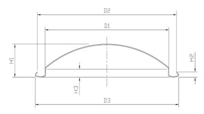
The outer diameter of the flange (D3) is 72.35±0.25mm Inner diameter of flange (D2) 70.00±0.25mm Flange height (H2) 2.50±0.2mm Buried depth (H3) 3.10±0.15mm Fit diameter (D1) 62.80±0.20mm Dry glue quantity 70-90mg Deformation pressure ≥ 1.8MPa Burst pressure ≥ high pressure 2.1MPa Indenter fits well with the company's indenter Sheet thickness 0.4 Iron hardness T4CA
