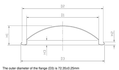
Inner diameter of flange (D2) 70.00±0.25mm Flange height (H2) 2.50±0.2mm Buried depth (H3) 3.10±0.15mm Fit diameter (D1) 62.80±0.20mm Dry glue quantity 70-90mg Deformation pressure ≥ 1.8MPa Burst pressure ≥ high pressure 2.1MPa Indenter fits well with the company's indenter Sheet thickness 0.4 Iron hardness T4CA
