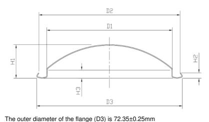
Inner diameter of flange (D2) 70.00±0.25mm
