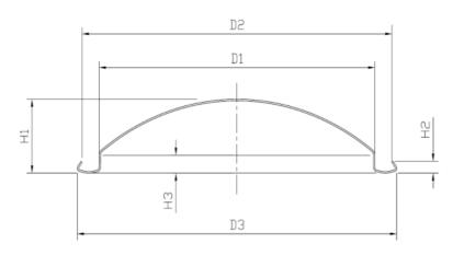
The outer diameter of the flange (D3) is 72.35±0.25mm Inner diameter of flange (D2) 70.00±0.25mm Flange height (H2) 2.50±0.2mm Buried depth (H3) 3.10±0.15mm Fit diameter (D1) 62.80±0.20mm Dry glue quantity 70-90mg Deformation pressure ≥ 1.8MPa Burst pressure ≥ high pressure 2.1MPa Indenter fits well with the company's indenter Sheet thickness 0.4 Iron hardness T4CA
