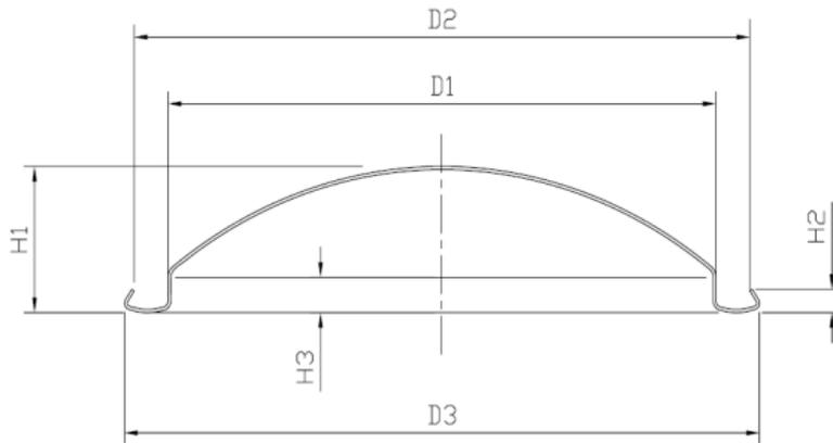
The outer diameter of the flange (D3) is  $72.35 \pm 0.25$ mm
