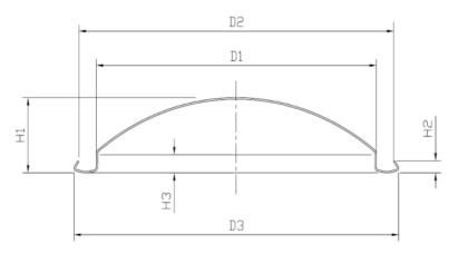
The outer diameter of the flange (D3) is 72.35±0.25mm Inner diameter of flange (D2) 70.00±0.25mm Flange height (H2) 2.50±0.2mm Buried depth (H3) 3.10±0.15mm Fit diameter (D1) 62.80±0.20mm Dry glue quantity 70-90mg Deformation pressure  $\geq$  1.8MPa Burst pressure ≥ high pressure 2.1MPa Indenter fits well with the company's indenter Sheet thickness 0.4 Iron hardness T4CA
