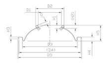
Flange diameter (D5) 69.90±0.25mm Inner diameter of flange (D4) 67.80±0.25mm Flange height (H3) 2.45±0.15mm Buried depth (H4) 5.10±0.10mm
