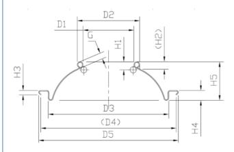
Inner diameter of flange (D4) 55.70±0.20mm Flange height (H3) 2.20±0.15mm Buried depth (H4) 4.70±0.15mm Total height (H5) 13.50±0.15mm Contact height (H1) 4.00±0.10mm Fit diameter (D3) 48.00±0.20mm Outer diameter of tank mouth (D2) 31.20±0.10mm Inside diameter of tank mouth (D1) 25.40±0.10mm Dry glue quantity 50-70mg Deformation pressure ≥1.3MPa Bursting pressure ≥1.5MPa Indenter fits well with the company's indenter
