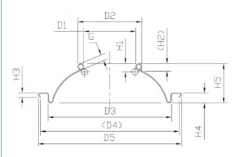
Flange diameter (D5) 57.60±0.20mm Inner diameter of flange (D4) 55.70±0.20mm Flange height (H3) 2.20±0.15mm Buried depth (H4) 4.70±0.15mm Total height (H5) 13.50±0.15mm Contact height (H1) 4.00±0.10mm Fit diameter (D3) 48.00±0.20mm
