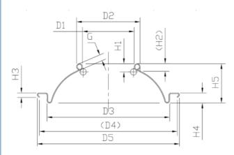
Flange diameter (D5) 57.60±0.20mm Inner diameter of flange (D4) 55.70±0.20mm Flange height (H3) 2.20±0.15mm Buried depth (H4) 4.70±0.15mm Total height (H5) 13.50±0.15mm Contact height (H1) 4.00±0.10mm Fit diameter (D3) 48.00±0.20mm Outer diameter of tank mouth (D2) 31.20±0.10mm Inside diameter of tank mouth (D1) 25.40±0.10mm Dry glue quantity 50-70mg Deformation pressure ≥1.3MPa Bursting pressure ≥1.5MPa Indenter fits well with the company's indenter
